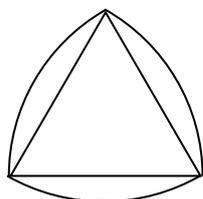
*This shape is also used for drills that drill “square” holes (almost square – the corners aren’t quite right).*
