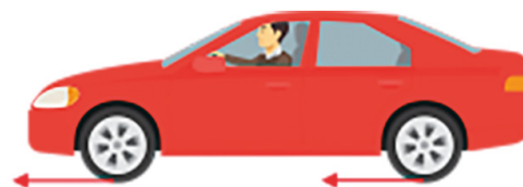
Fig. 1: The ground obligingly exerts an external, frictional force on the car that pushes it forwards (similarly at all four wheels, even if the car isn't '4-wheel drive').
