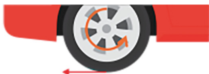
Fig. 3: If the car is driving to the left, the wheel must be rotating anticlockwise, which means that the bottom of the tyre is pushing on the ground to the right. Friction from the ground resists this by pushing to the left, moving the car forwards.
