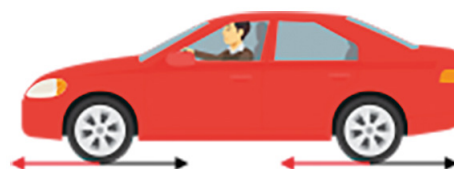
Fig. 7: The car wheels push on the ground (black arrows) and the ground responds by exerting a force on the car (red arrows) that pushes it forwards (similarly at all four wheels).
