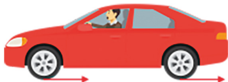
Fig. 2: On a very icy surface, the wheels are locked and sliding forwards, and friction now slows the car down (similarly at all four wheels).
