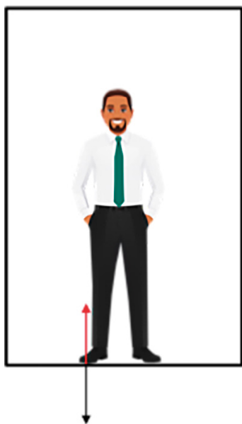
Fig. 10: A pair of equal and opposite contact forces at the bottom of a lift (elevator). Neither of these forces is the person's weight.
